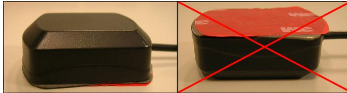
Figure 44 Correct GNSS antenna mounting
