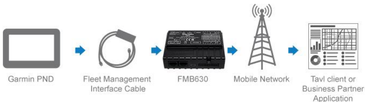
Figure 119 FMB630 +Garmin operational scheme
