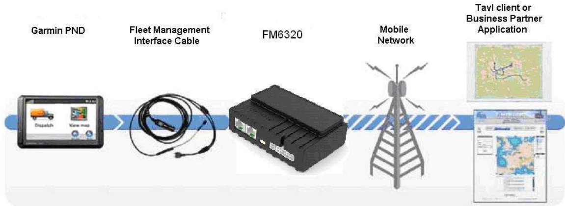
Figure 116 FM6320+Garmin operational scheme
