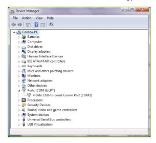
Note: Remember this Com number. It needs to be input into the MEITRACK Parameter Editor. It is COM3 in this example and it would be COM4 or COM5... in your computer.
