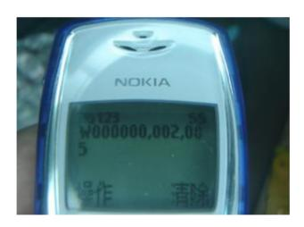
Step2. VT300 will send back one SMS-----Set Time (preset time interval) OK.
