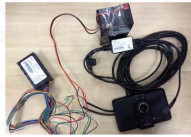
Figure 18. GV300 connection with Garmin GPS set
