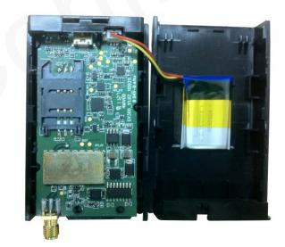
Figure 6. Backup Battery Installation There is an internal backup Li-ion battery,
