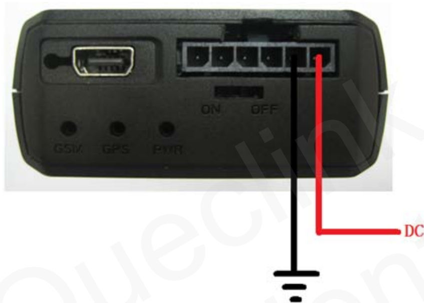
Figure 8. Typical Power Connection
