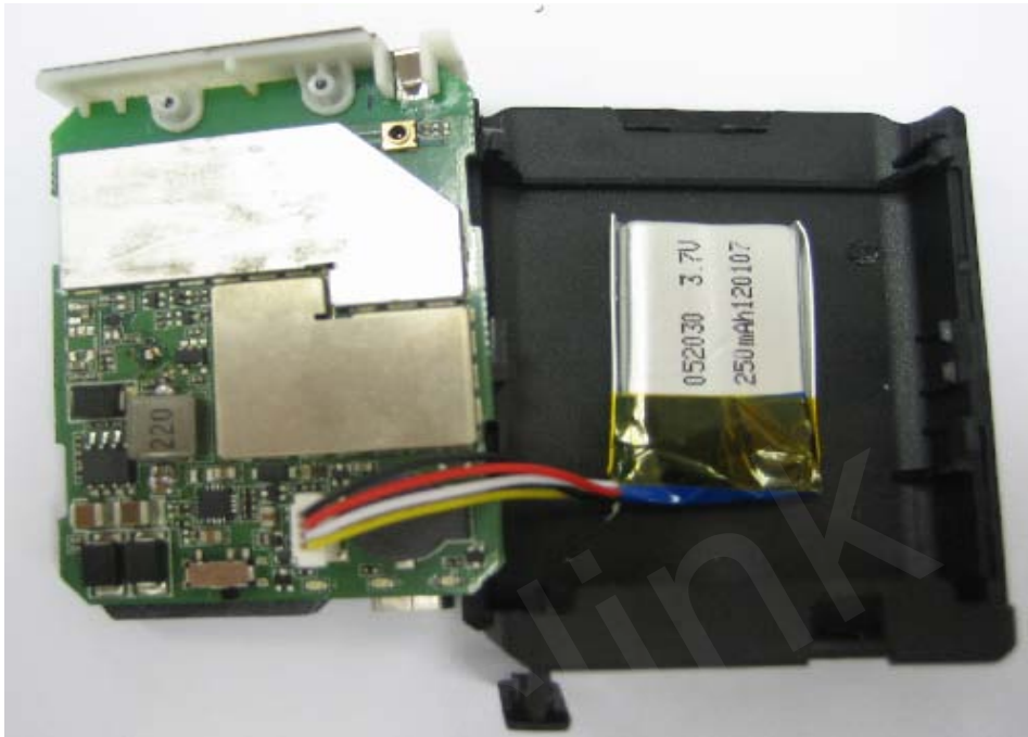
Figure 6. Backup Battery Installation
