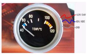
Connect fuel sensor or temperature sensor refer to above picture.
