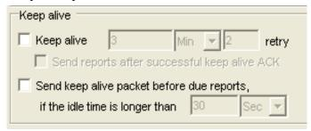
Parameters: On/Off, and interval / retry times. In order to keep connection in GPRS network, the unit can be set to send short keep alive report to the server in order to prevent the disconnection from the mobile service provider.
