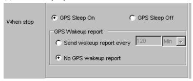
While the device is in stop status, user can let the GPS go to sleep mode for power saving. If select GPS Sleep ON, user can setup the wakeup report configuration/ or NO GPS wakeup report.
