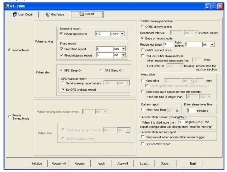
Report setup can be configured in this section. To activate the function(s), please select " $\sqrt{}$ " in checkbox and fill in data in the textbox. There are 2 modes for the GT2000NP/GT2500NP, first is the Normal mode, and second is the Power saving mode. In normal mode, the GPS will be always activated if GT2000NP/GT2500NP is in moving state. However, if in Power saving mode, GT2000NP/GT2500NP will turn off the GPS power if there is no report to send.
