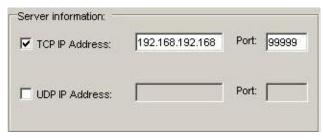
TCP/UDP address and Port number of alarm center being set, UNIT will send message to these address. Note that either TCP or UDP should be selected.
