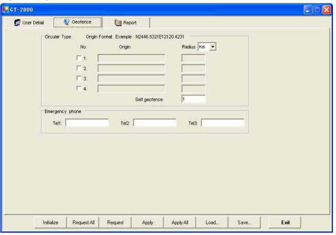
Setup the circular Geofence parameters in this window. The format will be center of the Geofence and the related radius.
