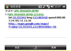
\*When lost fix to satellites, it will track by LBS / CELL-ID. And the SMS will include two positions: - GPS coordinates of the last known position. -LAC code. Open www.gpstrackerxy.com find "manual track", and put the received code in LAC and Cell-ID fields to location by LBS technology.
