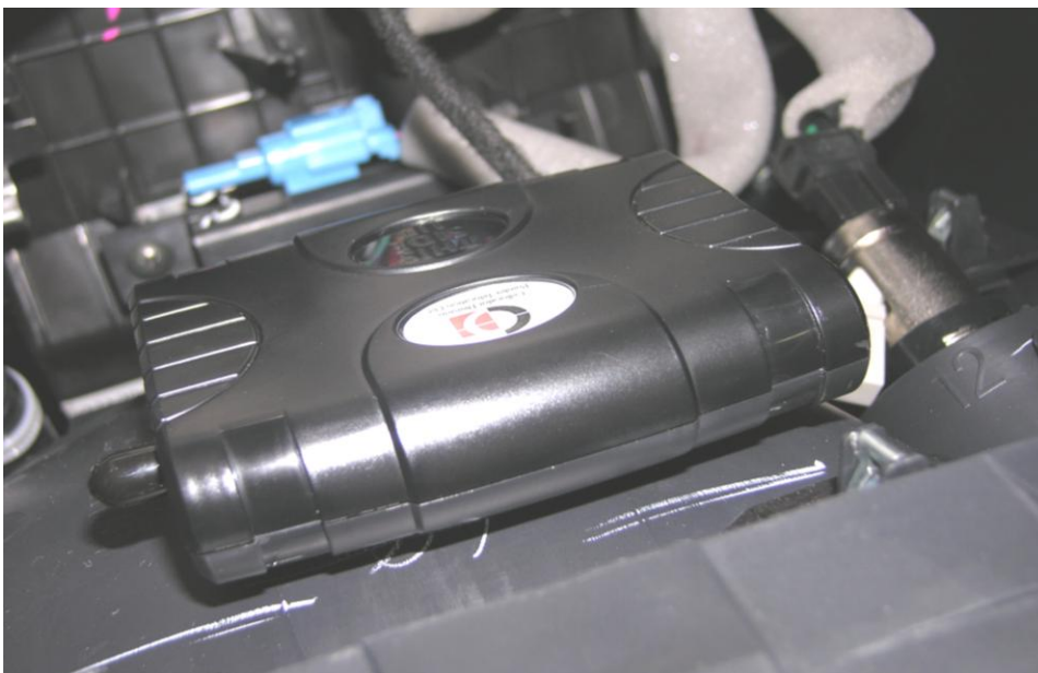
Figure 14: Ensuring the device is located with 30cm free radius
